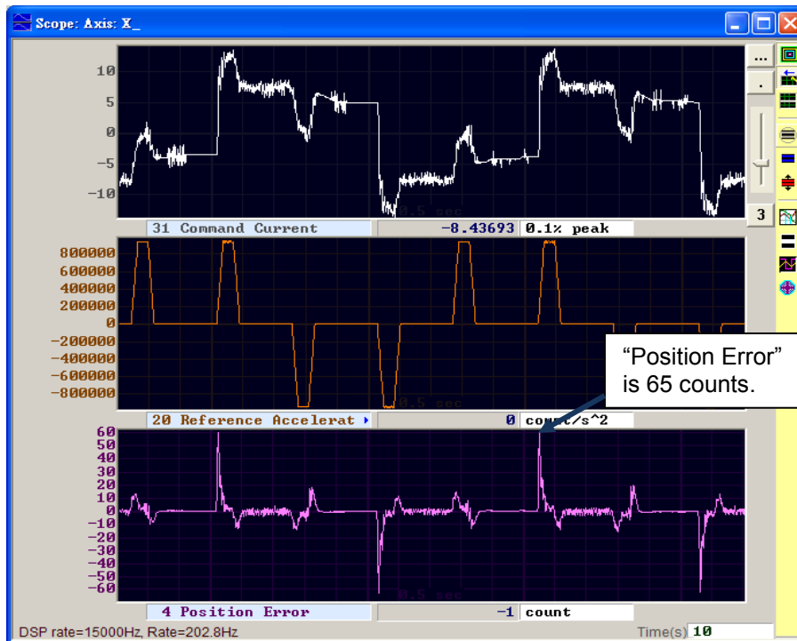
Figure6.6.2.4 Result of adding acceleration feed-forward
